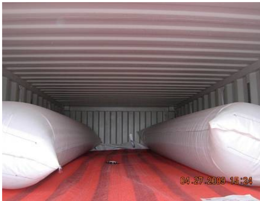
Photo #10 Pneumatic Dunnage
