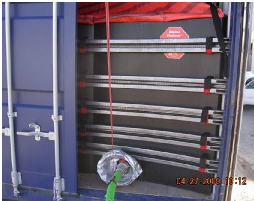
Photo #6 5,300 US Gallons Being Added to the Big Red Flexitank™
