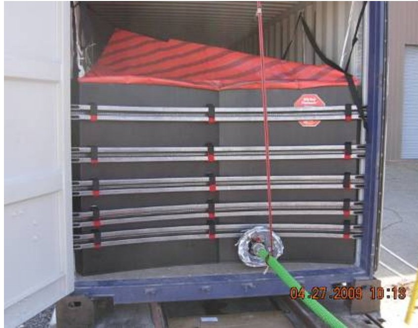
Photo #5 Flexitank Ready for Water
