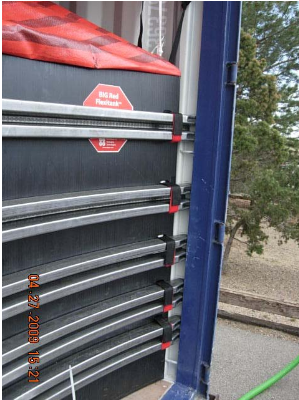
Photo #11 Bulkhead Interface to Bull Board Slots
