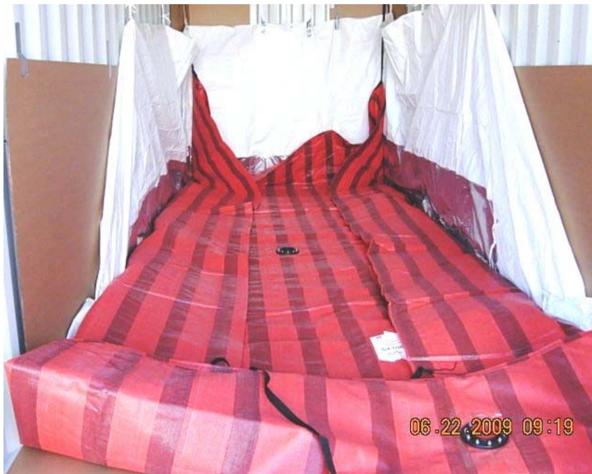
Photo # 2 Flexitank Installation
