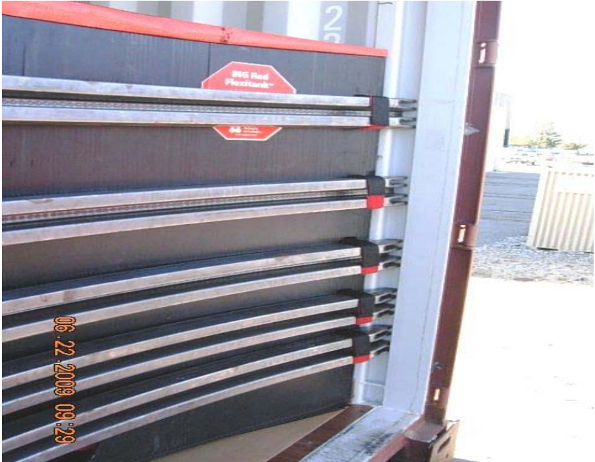
Photo #4 Bulkhead Installation
