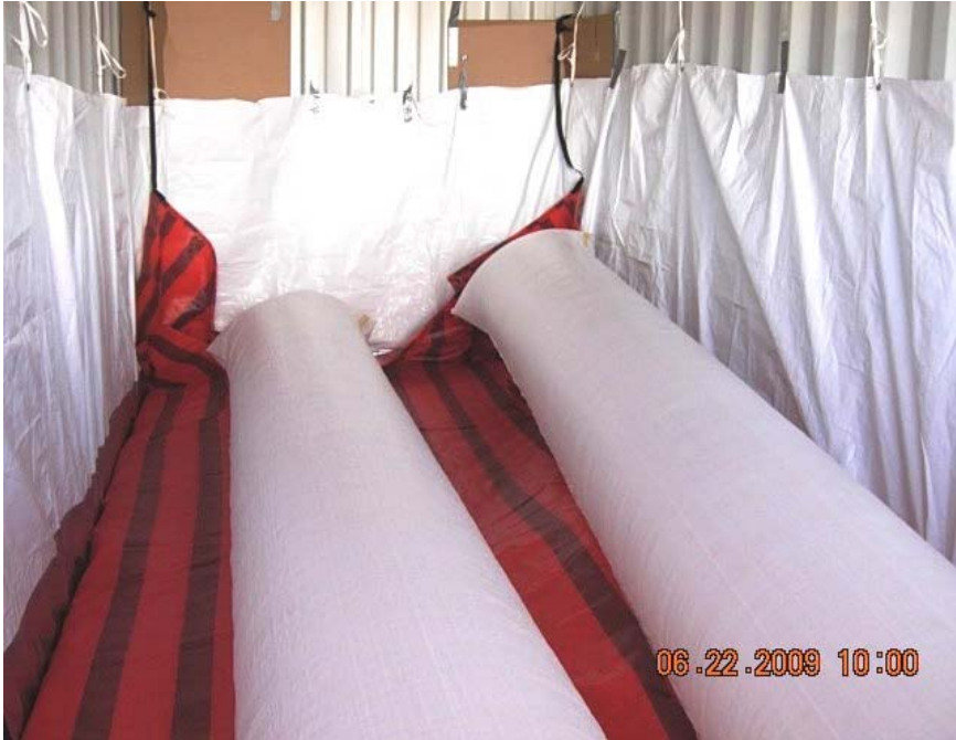
Photo #5 Pneumatic Dunnage Installation
